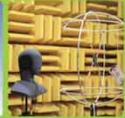
Semi-anechoic chamber According ISO 3744 According ISO 3745 According ISO 7779
